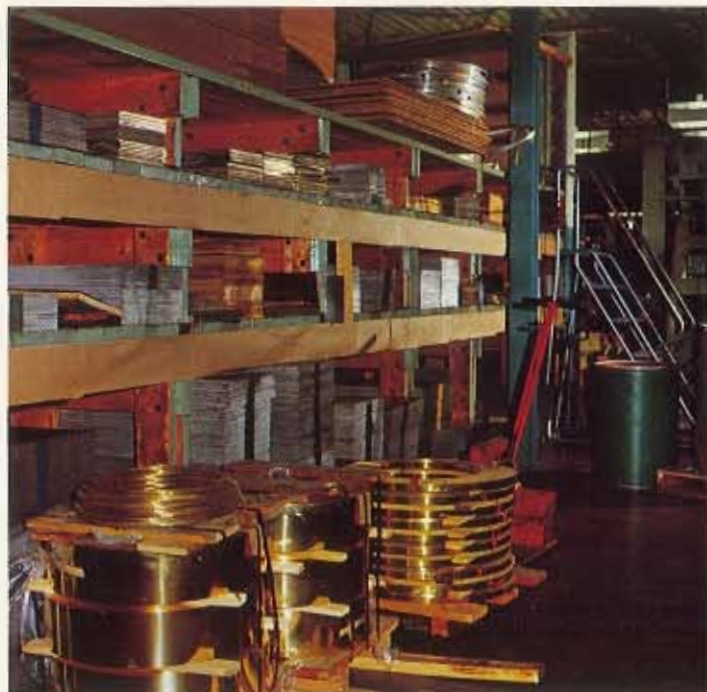
Knives begin as sheets and coils of steel, brass, and nickel silver.
