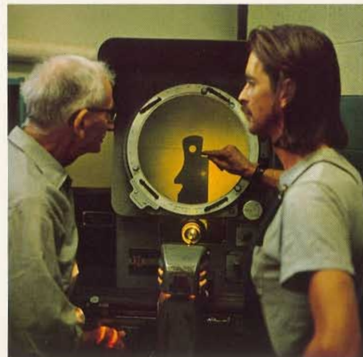
Inspecting enlarged image of part with optical comparator.
