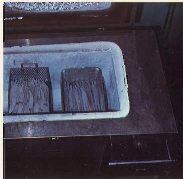
Freezing: Hardened blades frozen to minus 125°F.
