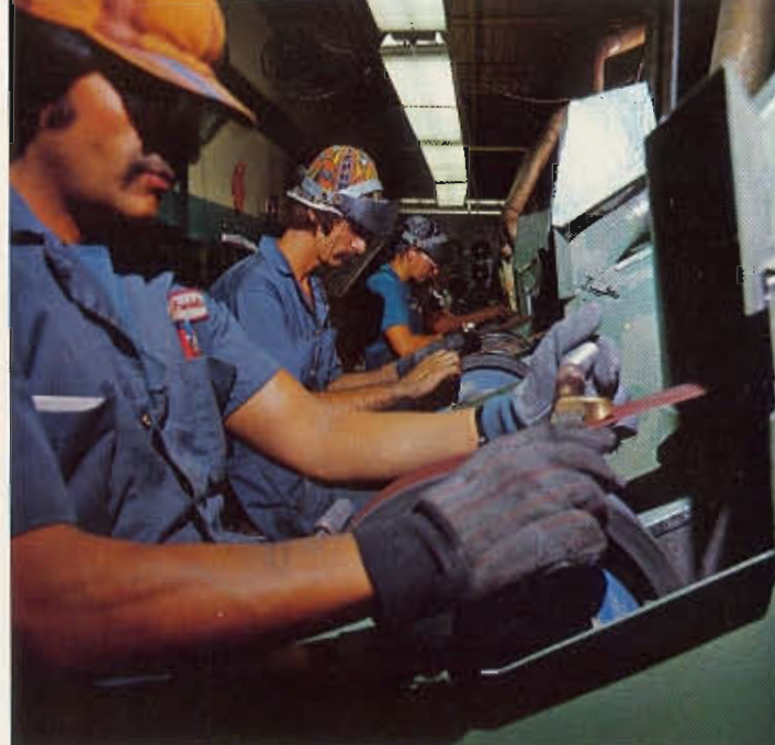
Hafting line, where knife handles are shaped on coated abrasive belts.
