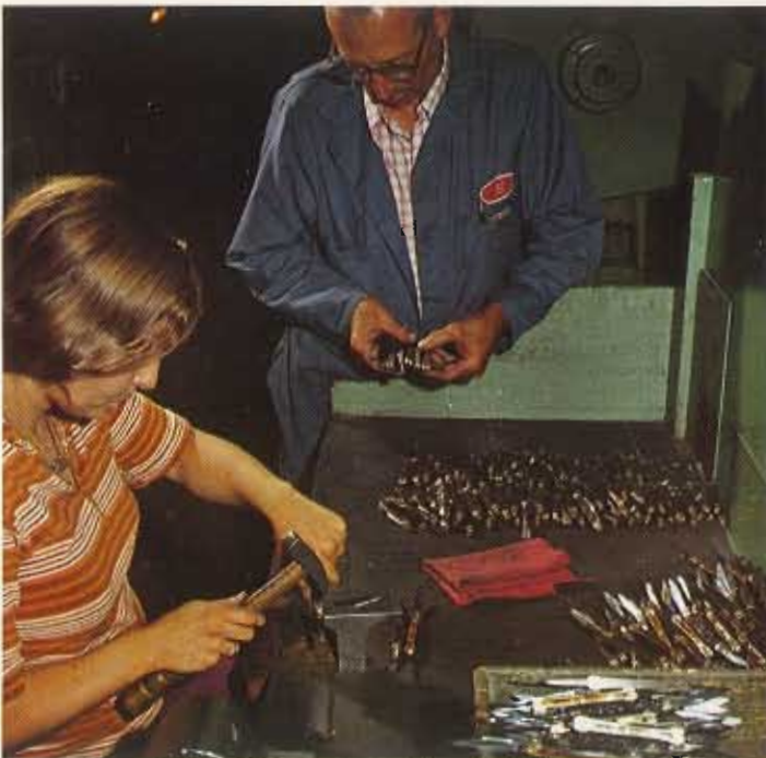
Adjusting pocket knife blades to "walk and talk."
