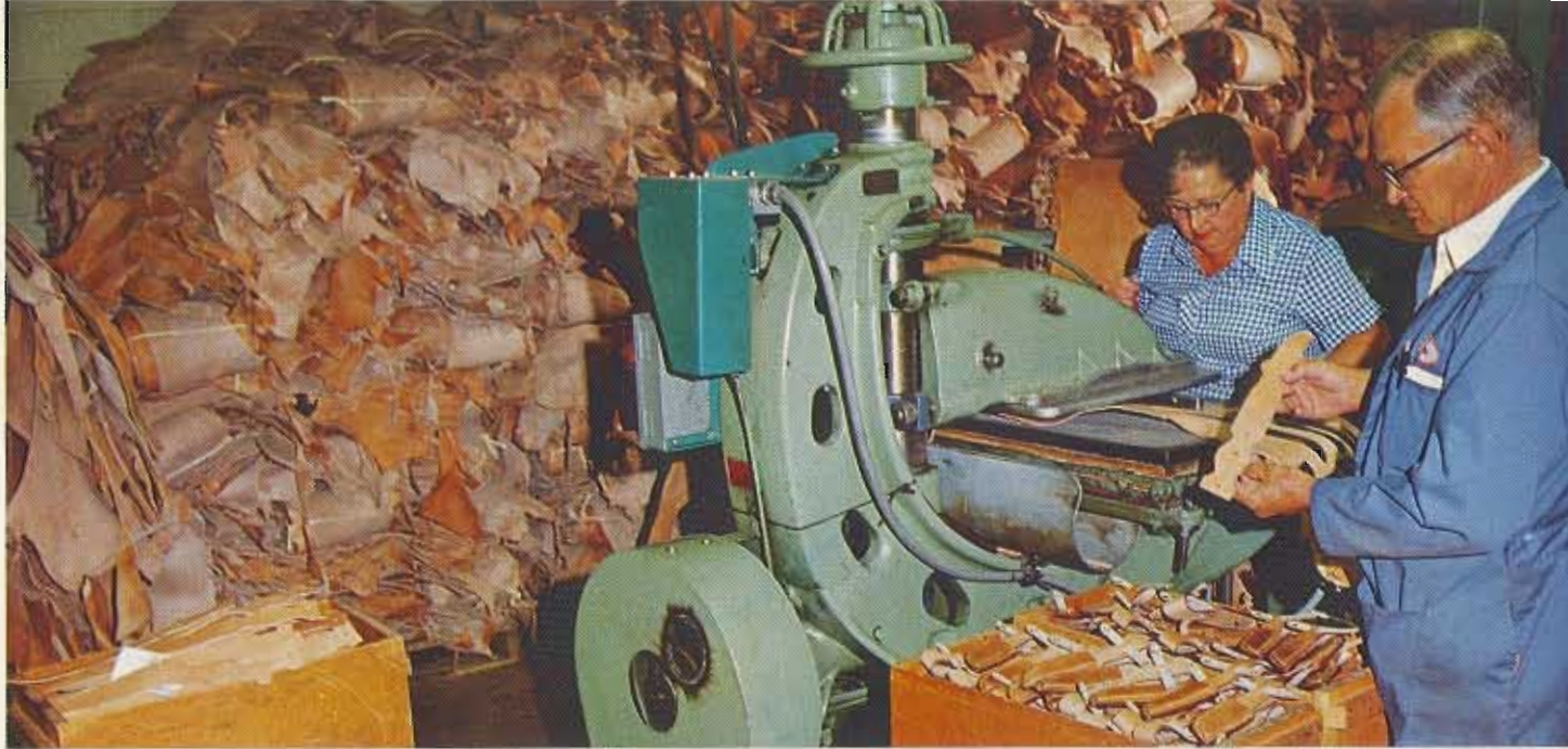
Cutting sheath parts from steer hide on a "clicker" machine.
