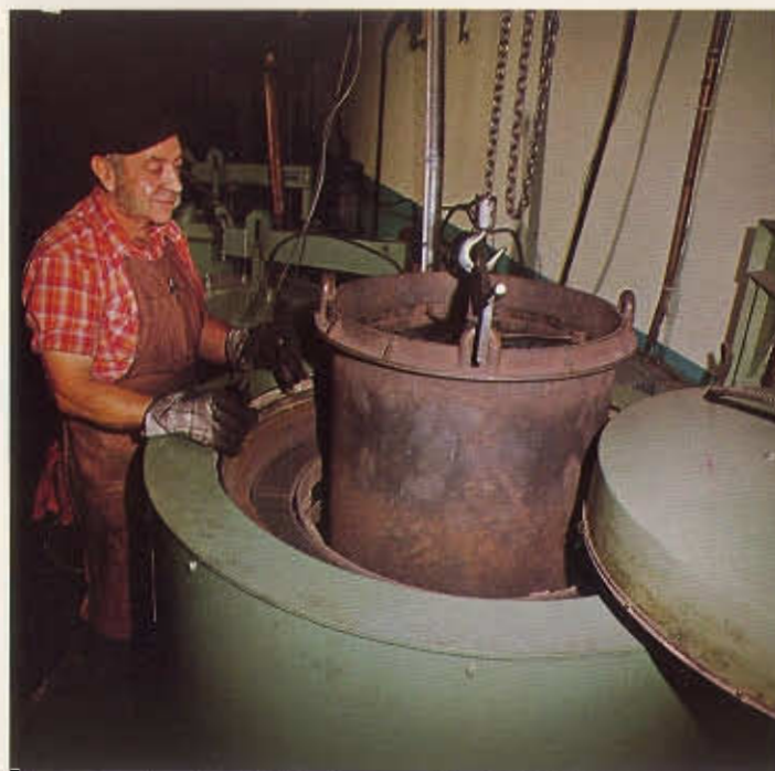
Tempering: Loading electric furnace with pot of hardened blades.
