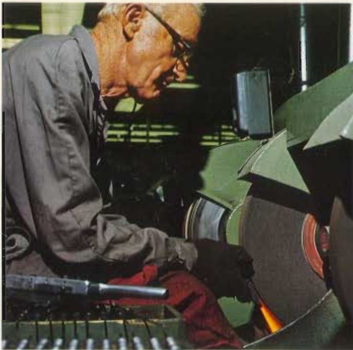
Dressing pocket knife parts on a grindstone.
