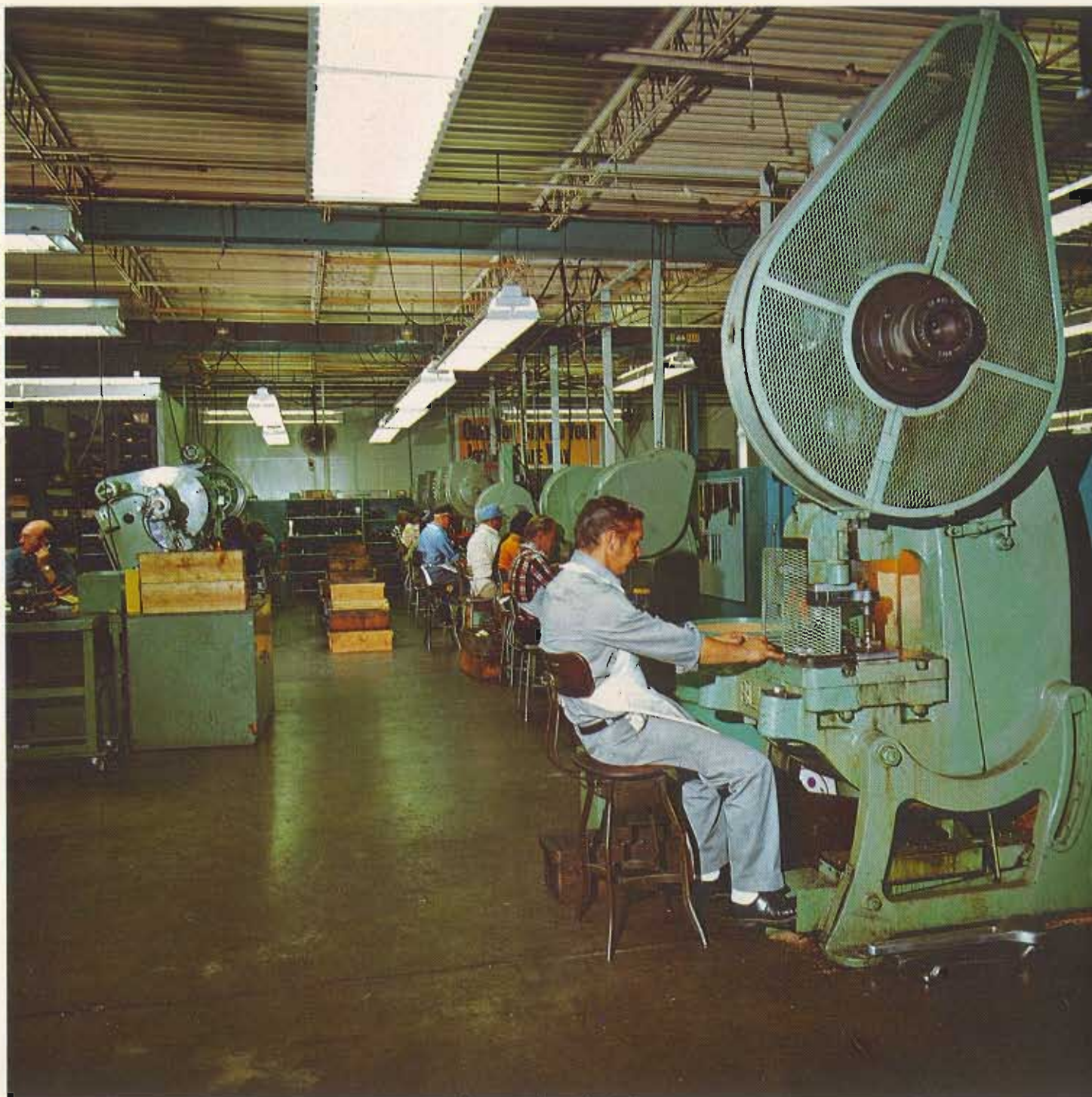
Part of the press room with double row of small presses for light stamping and piercing.
