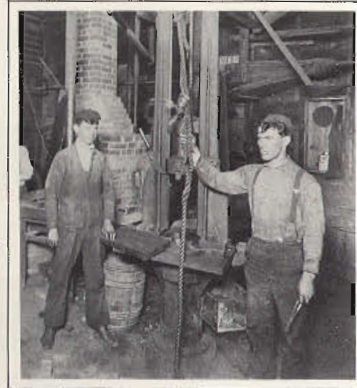
Drop hammer in forge room, C. Platts and Sons Cutlery Co. This part of plant had a dirt floor, and drop hammers were set on ends of large logs em- bedded deep in the ground. Note bellows over the head of man on right.
