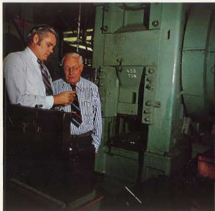
A 400-ton mechanical press has replaced the drop hammers of the past.
