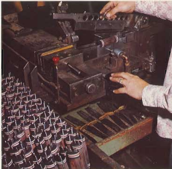
Fitting handle on tang end of blade.
