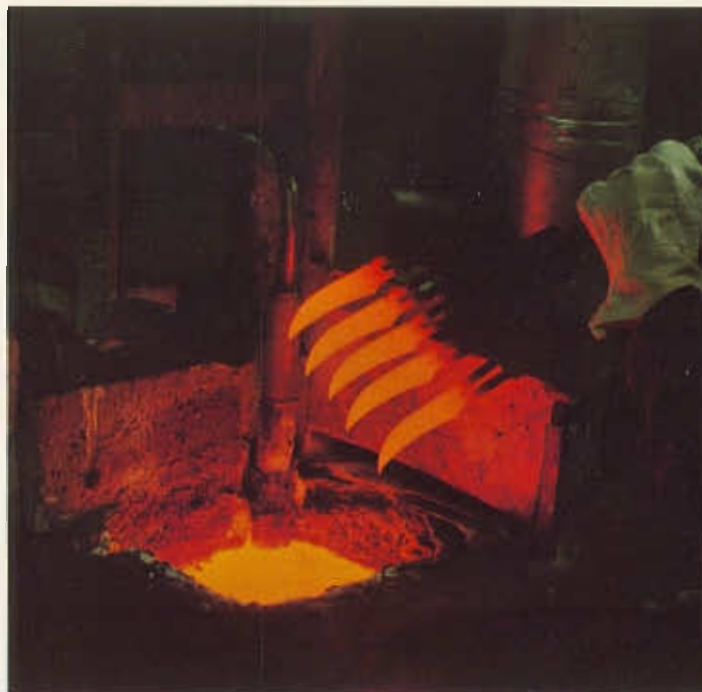
Hardening: Blades at high temperature leave furnace for oil quench.
