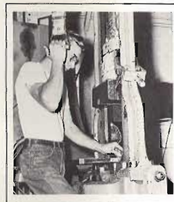
Making pocket knife bolsters on one of the drop hammers at the old Western States plant.
