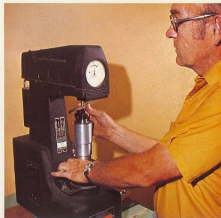
Quality control: One of many tests is measurement of Rockwell hardness.
