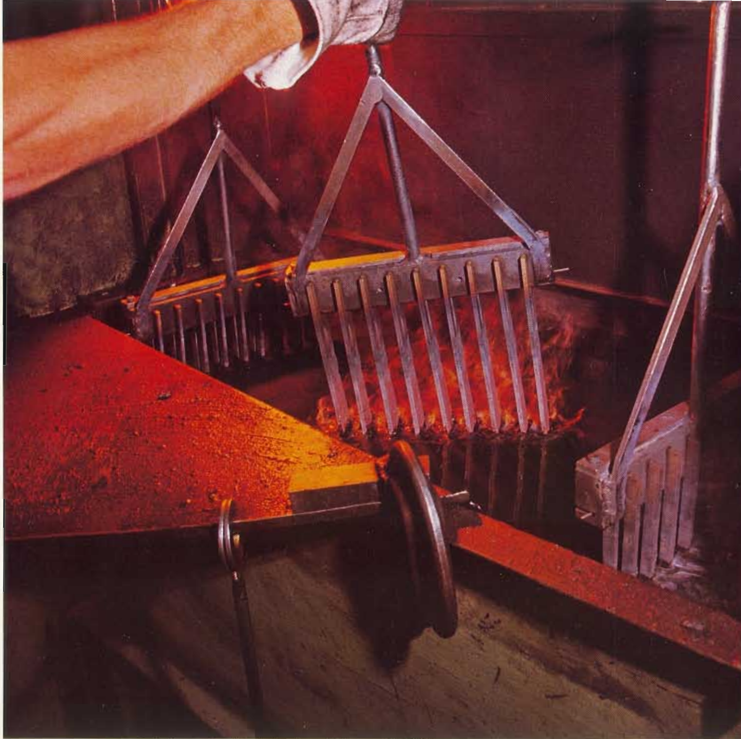
Quenching: Heated knife blades become hard steel when plunged into special oil bath.
