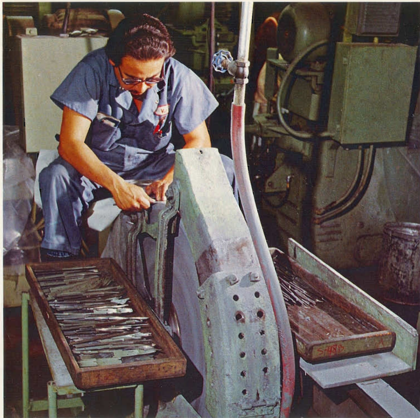
The old skill of free-hand grinding on large-diameter stones is still an important part of crafting fine knives.
