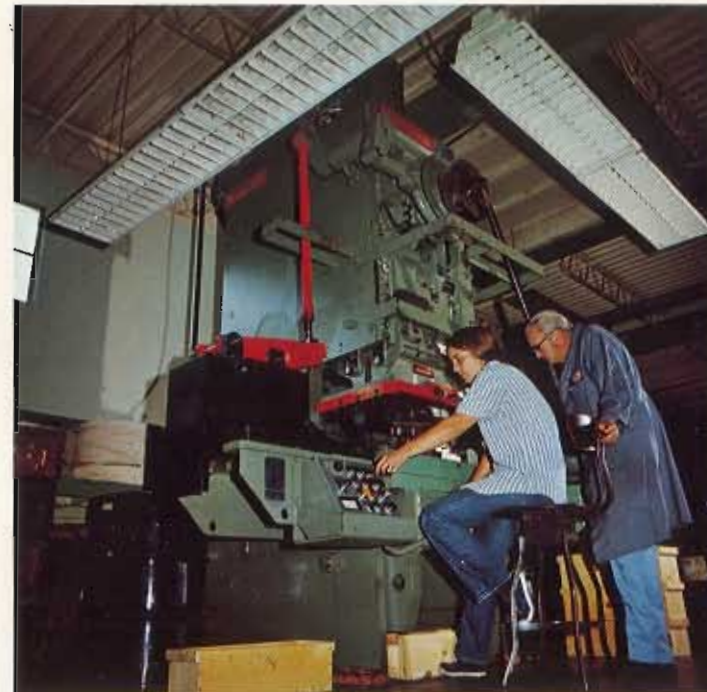
A 90-ton press with automatic feed cuts knife blanks from steel strip.
