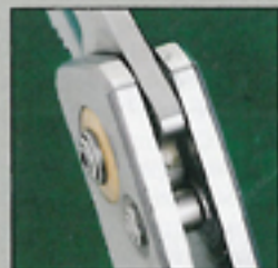
The P.A.L.™ lock's shouldered hardened steel piston is offset to provide tight lockup with all play eliminated.
