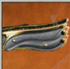
Winged scales are 6061 T6 aluminum, hard anodized. The 7402GK frame is gold titanium nitride coated.
