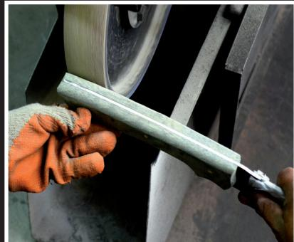
**HIGH IMPACT POLYPROPYLENE HANDLES** are strong and indestructible. These handles are molded directly to our machetes and knives blades making them impossible to separate. The tang on our polypropylene handle continues to the back of the handle, with a metal lanyard passing through it for added strength.
