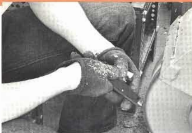
Knives are glazed, scoured and hand-buffed to remove rough areas.
