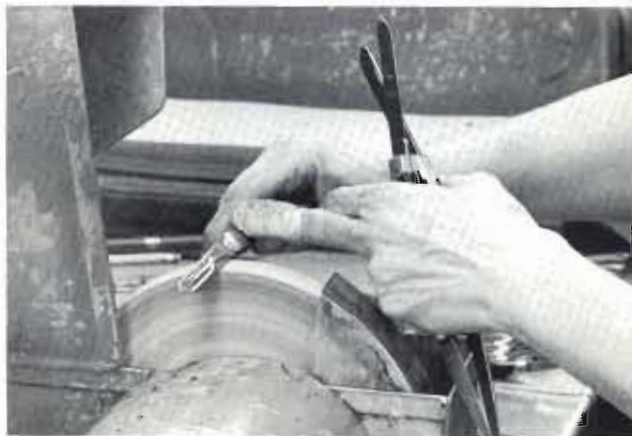
Blades are sharpened to specified cutting edge.
