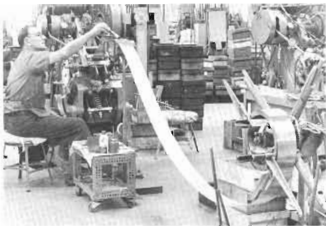
Stamping out brass linings, blades, center scales, etc.
