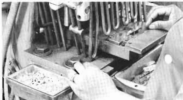
Bolsters and liners are riveted together in position . . . ready for cover.
