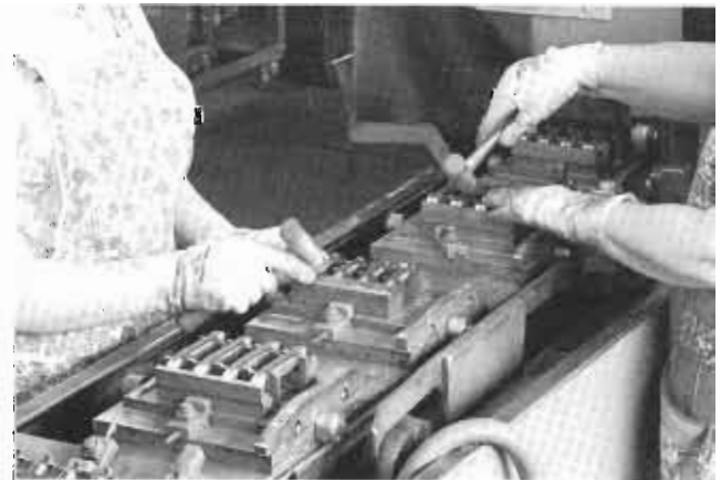
Loading assembled knives into machine for grinding and polishing of spring backs.
