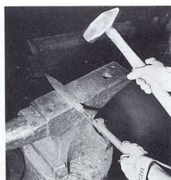
Forging a blade.
