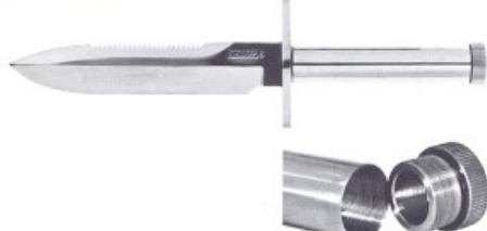
**"ATTACK-SURVIVAL"**—5½" and 7½" blades of ¼" stock. Sawtooth edge on top. 1" stainless steel tubular handle, silver-soldered to ¼" oblong brass hilt, fitted with removable, threaded brass butt cap and waterproof "O" ring. (See detail above.) Flared holes in top and bottom of hilt accommodate wrist thong and facilitate attachment of rod for conversion to spear. (Name etching only extra feature available. Manual for combat use available. See Page 21.)
