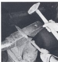
Forging a blade.
