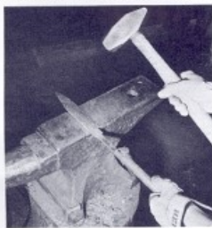
Forging a blade.
